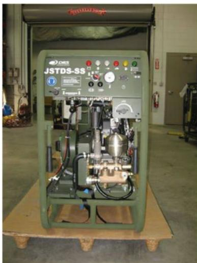
**Joint Service Transportable Decon System Small Scale
